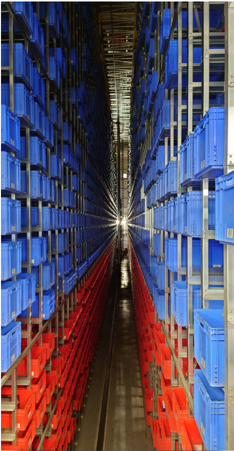
High-bay warehouse with double storage locations is precisely controlled by Delphi programs
